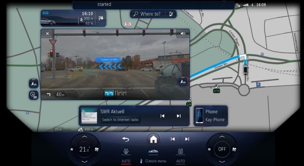
B. MBUX Augmented Reality navigation view in MBUX Media display.
